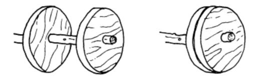
Fix wooden wheels to the aid with nuts and bolts, screws or an axel.
